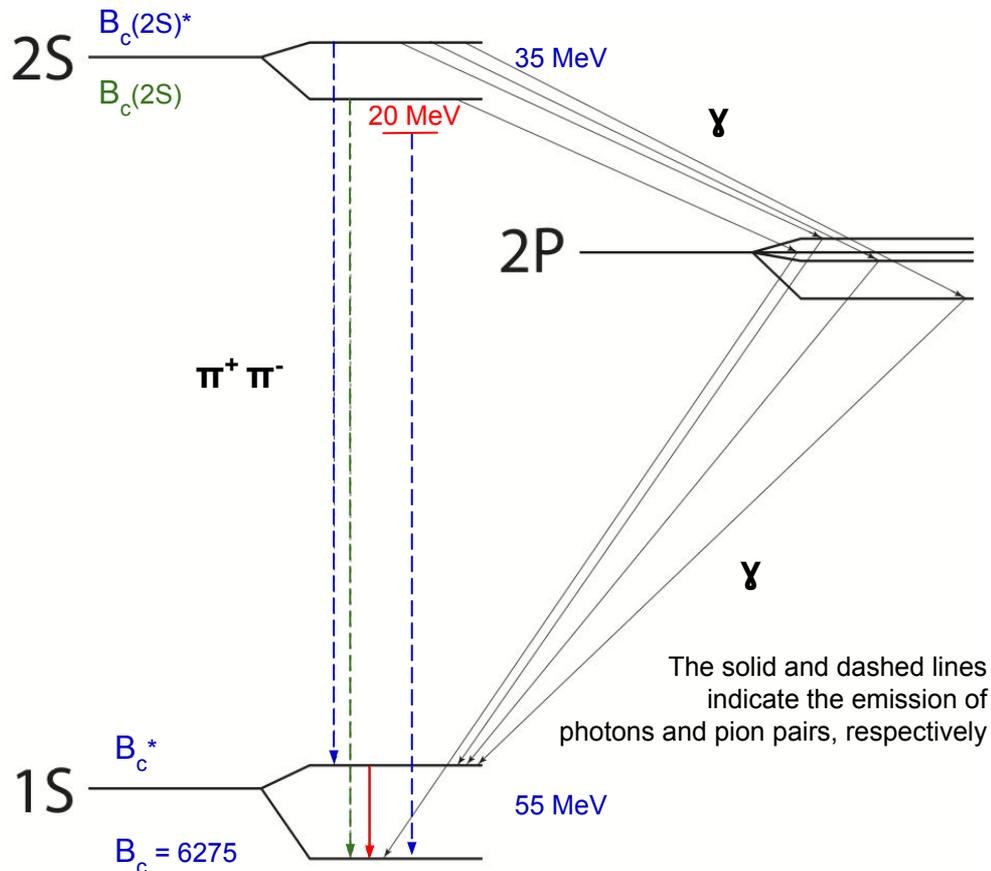
The solid and dashed lines indicate the emission of photons and pion pairs, respectively
