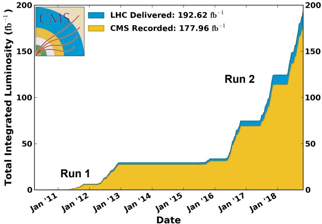
CMS has recorded  $\sim 5$  fb<sup>-1</sup> at  $\sqrt{s}=7$  TeV,  $\sim 20$  fb<sup>-1</sup> at  $\sqrt{s}=8$  TeV, and  $\sim 140$  fb<sup>-1</sup> at  $\sqrt{s}=13$  TeV of data for physics analysis
