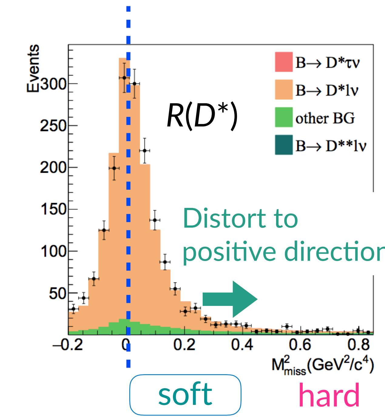
Soft emission distorts around the center of the missing mass dist.
