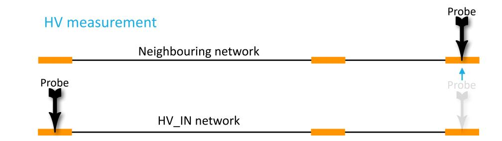
Probe on primary pad doesn't move, secondary probe moves to the pad in the neighbouring network. Start HV measurement.
