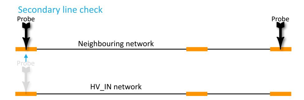
Probe on secondary doesn't move, move probe from primary pad in HV network to some other pad in neighbouring network. Measure resistance.
