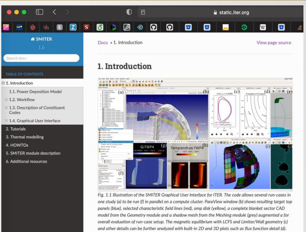
Triangular meshes (j) are the main run-case geometry setup (e) that are directly imported or meshed from CAD models (i) defeatured to retain only the required PFC surfaces for meshing with different algorithms and hypotheses. Resulting heat fluxes on the panels (g) can be further processed to get ITER first wall panel (FWP) (h) using FEM thermal models built into the SALOME environment of normal heat flux (NHF) or enhanced heat flux (EHF) cooling sub-structures.
