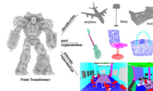
Figure 1. The Point Transformer can serve as the backbone for various 3D point cloud understanding tasks such as object classification, object part segmentation, and semantic scene segmentation.
