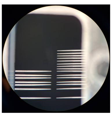
Speck on one of the needles successfully removed using a probe needle
