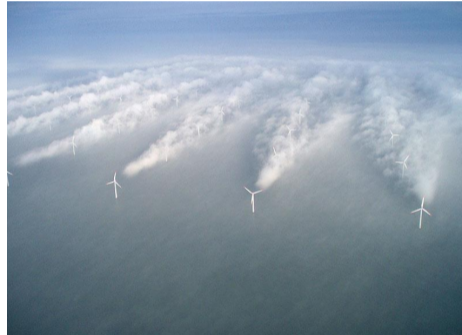
Wake turbulence behind individual wind turbines
