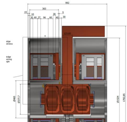
Preliminary design of a muon cooling cell → Demonstrator
