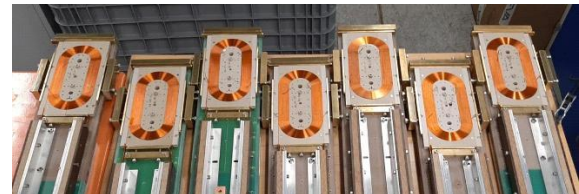
ReBCO Racetracks, CERN
